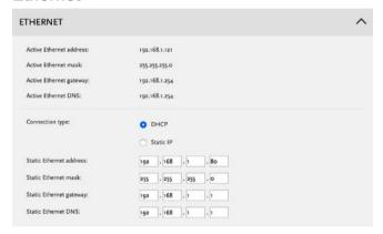
Allows you to change the Ethernet configuration. Note that incorrect settings may make the 251 unreachable via the web page.
