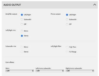
**Amplifier output** and **Phono output**: Can be independently set to **Left/Right**, corresponding to the main left and right channels, **Subwoofer**, corresponding to the subwoofer(s), or **Off**, to switch the corresponding output off.
