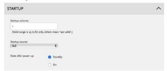
**Startup volume**: Specifies the initial volume for the analogue outputs and, if the 251 is a Controller, sent on Meridian Comms for other connected products. The start volume is set when the 251 is first powered up, and a few seconds after going into standby.
