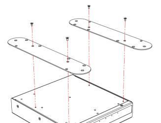
The kit consists of two plates and four screws, allowing the 251 Powered Zone Controller to be mounted in either of two orientations, as shown in the following diagrams:
