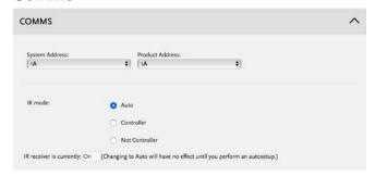
**System Address**: If an installation contains multiple zones that are connected together with Meridian Comms, each one needs a different System Address if they are to have independent source selection and volume controls. If the installation uses LAN connections then this can be left at its default. **1A**.
