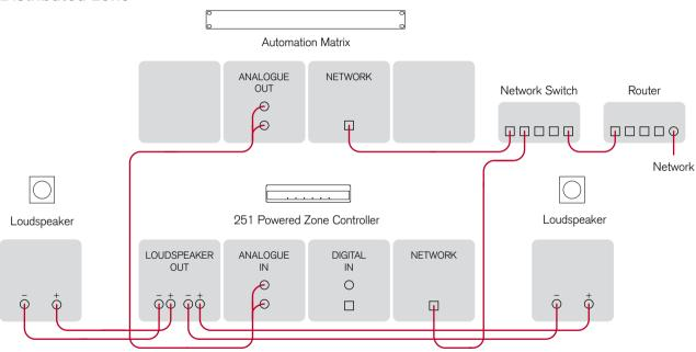
This layout is intended to play back audio in a single zone as part of a larger, whole-house, automation system. The 251 is located in a central rack along with the automation system's audio matrix
