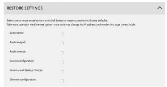
Allows you to restore one or more groups of settings to their factory defaults. Note that restoring the Ethernet settings will enable DHCP, which may change the IP address of the 251, and you may have to find the new address as described below.
