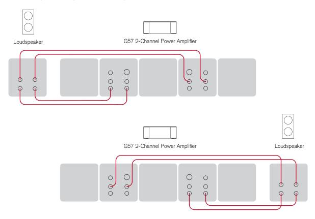
Extremely high sound quality can be achieved using two separate G57 Two-channel Power Amplifiers, one to drive each loudspeaker. The two channels in each G57 Two-channel Power Amplifier are used to drive the LF and HF units in each loudspeaker.
