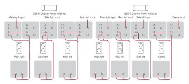
Two G55 Five-channel Power Amplifiers can be used as the basis of a superb seven-channel surround system, taking advantage of bridge mode operation to give more than twice the power output for the three front channels.
