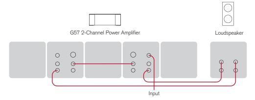
You can use the G57 as a mono power amplifier, to obtain more than twice the power output, by wiring it in bridge mode.
