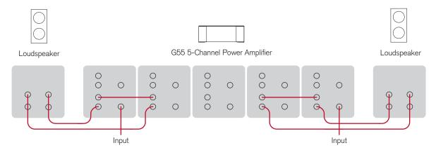
You can wire channels 1/2 and 4/5 in bridge output mode, to obtain more than twice the power output.
