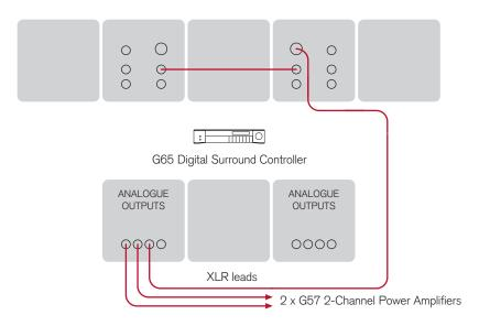
Three G57 Two-channel Power Amplifiers can be used in bridge mode for each of the front channels of a G65 Digital Surround Controller, which are provided as balanced outputs.
