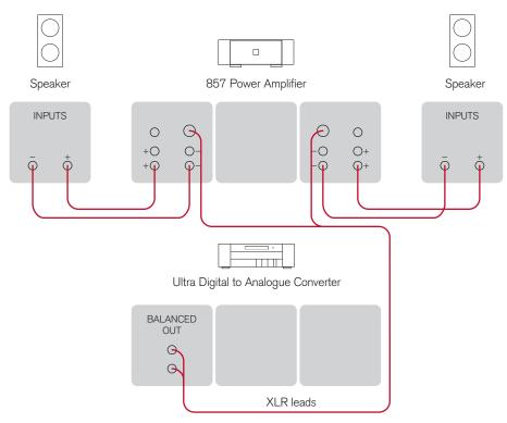
You can connect the Reference Two Channel Power Amplifier to a preamplifier with balanced outputs, such as the Meridian Ultra Digital to Analogue Converter.
