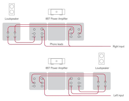
Extremely high sound quality can be achieved using two separate Reference Two Channel Power Amplifiers, one to drive each loudspeaker. The two channels in each amplifier are used to drive the LF and HF units in each loudspeaker.
