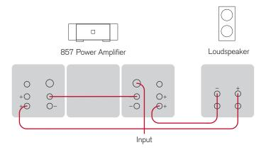
You can use the Reference Two Channel Power Amplifier as a mono power amplifier, to obtain more than twice the power output, by wiring it in bridge mode.
