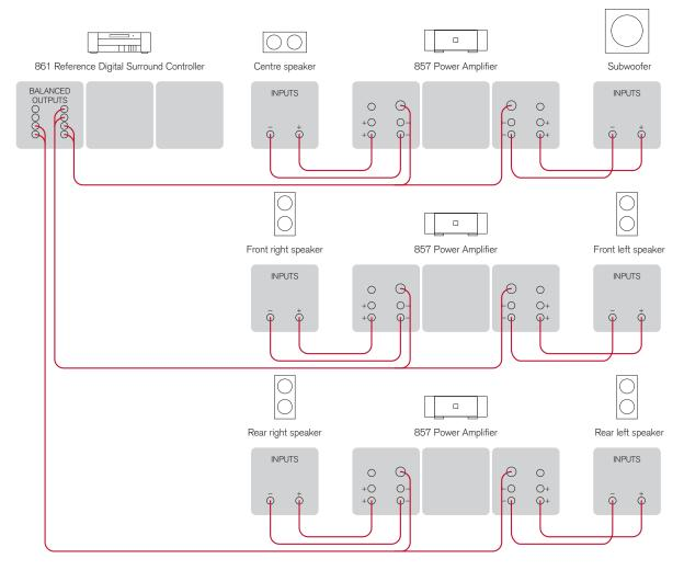
You can use three Reference Two Channel Power Amplifiers to drive the five loudspeakers and subwoofer in a surround system, using the six of the balanced outputs available on the OA18 cards.
