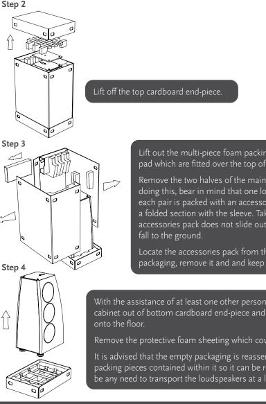
Lift out the multi-piece foam packing and flat foam pad which are fitted over the top of the cabinet.
