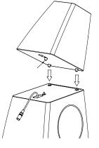
Hold the head-unit at a slight forward angle above the main cabinet and lower it carefully, so that the front two spike-cups fit over the front two spikes on the main cabinet. Carefully lower the rear of the head-unit so the rear spike-cup locates onto the rear spike.
